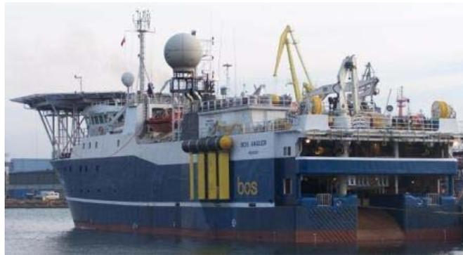
Following a successful upgrade the BOS Angler is equipped for multiple streamer surveys and prepared for OBS and other seabed operations. BOS Angler is a DP II Ice Class survey vessel and is already attracting interest for work in Arctic and other northern exploration latitudes.
